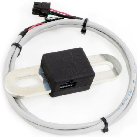
Figure 1-10 EMUS G1 Dual Range Current Sensor: Bus Bar type
