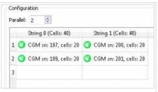
BMS Control Panel CAN devices configuration page: Configuration table with four CAN cell Group Module entries, after the configuration has been successfully committed and sent to BMS Control Unit. The green "check" icons indicate no errors.
